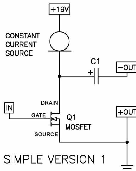
In this circuit we see a single gain element Q1, an N-channel power Mosfet. In the diagram you will see that the three pins on this device are labeled Source, Drain and Gate. The input signal comes to the Mosfet Gate pin, and the output signal appears at the Drain pin. The Source is attached to circuit Ground. This arrangement is known as "Common-Source" operation. Of the three possible ways of operating a Fet gain device, it is the one that offers both voltage and current gain.
