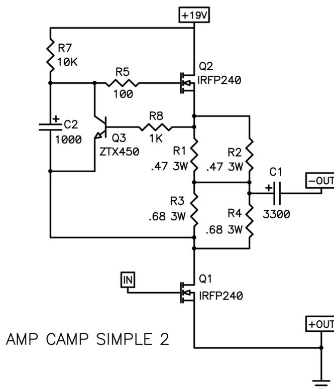
First we note that Q1 now actually has a part description IRFP240 which is a nice venerable power Mosfet which has been around for over 20 years. There is also Q2 which is the same type of Mosfet. Surrounding Q2 are several resistors, a small transistor Q3, and a capacitor. These elements are chosen to control Q2 in such a way that it acts as a DC constant current source which also varies AC-wise so as to favorably help the amplification provided by Q1.
